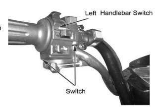
Insert connector of left handlebar switch into socket of main cable
