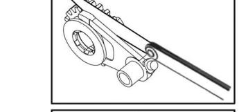
Measure shift fork groove width with vernier caliper
