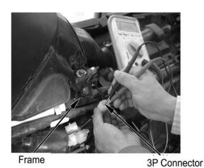
Make sure the yellow terminal of AC magneto 3P connector is not connected with frame body earth wire.
