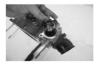
Compress the valve spring and remove valve cotter with tweezers.
