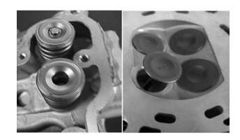
• Remove valve stem seal ring and valve lower seat.
