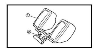
Check valve seat①, needle valve②, O-ring③ for damage, abnormal wear or dirt.
