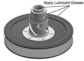
• Install guide pin and spacer ①
