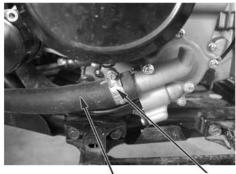
Water Inlet Hose, Engine Clamp
