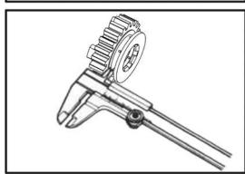
Measure shift fork thickness with vernier calipers;
