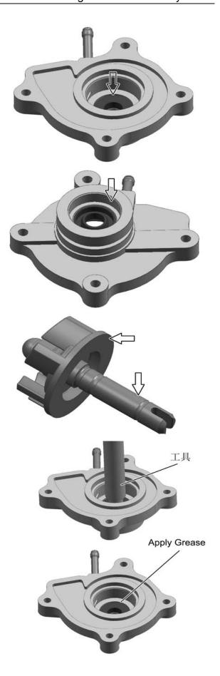
Install mechanical seal with a suitable socket wrench
