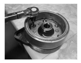
Check starter clutch roller and holder for abnormal wear or damage.
