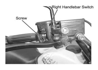
Insert connector of right handlebar switch into socket of main cable.
