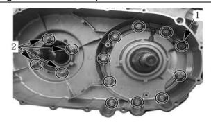
Remove dowel pin, front and rear gasket
