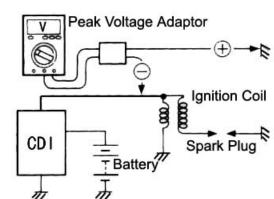
Set the multimeter to AC position
