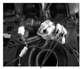
Connector, Handlebar Switch
