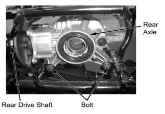
Remove nut and bolt of rear axle from frame.
