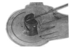
Install oil seal with special tool.
