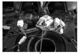
Connector, Handlebar Switch
