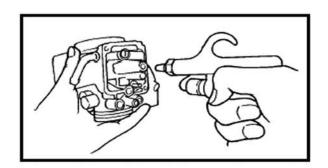
Check float (1), float tang (2) for damage.
