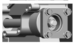
Apply sealant ①to the mating face of right crankcase.
