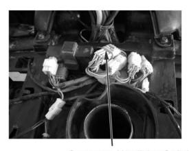
Connector, Handlebar Switch
