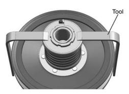
Tighten the ring nut with special tool to the specified torque.
