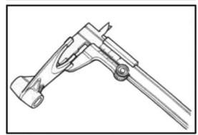
• Check shift fork ① and ② for damage or bend
