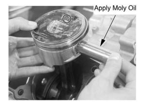
Place a clean rag beneath piston and install piston pin circlip ①
