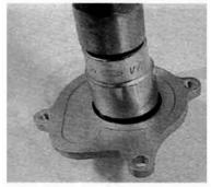
Install bearing with special tool
