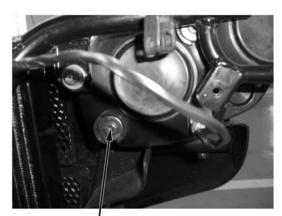
Adjusting Screw, Headlight Beam
