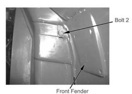
Remove screw for left side panel and footrest board
