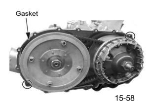
Install CVT case cover bolts and tighten diagonally in several steps.
