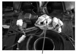
Connector, Handlebar Switch
