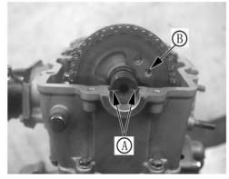
Recheck if the position of mark "A" and "C" is correct.
