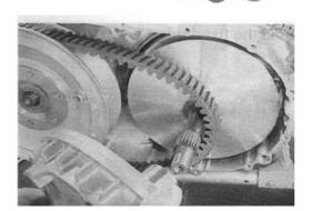
Tighten primary sheave nut with special tool to the specified torque;
