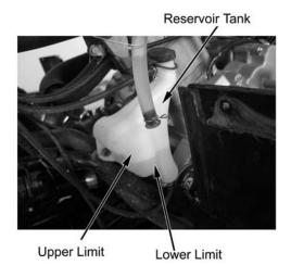
When the coolant level is below the LOWER limit, remove reservoir tank cap and add coolant till upper limit. (Add coolant or diluted original liquid).
