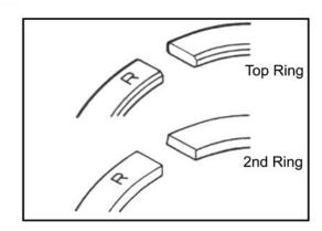
Position the gaps of the three rings as illustrated on the right. Before installing the piston into the cylinder, check that the gaps are so located.
