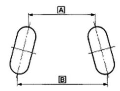
Toe-in out of the range:  $\rightarrow$  Adjust the locknut of tie-rod
