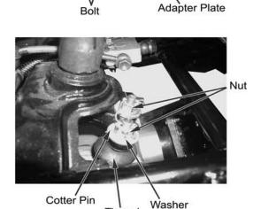
Remove fixing bolt of steering stem
