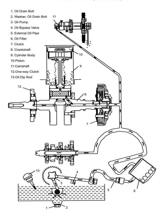
Inspection of Lubrication System ( $\rightarrow$ 11-8)
