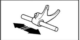
Put the guide bar on a flat plate and roll it. In case of any bend, replace with a new one.
