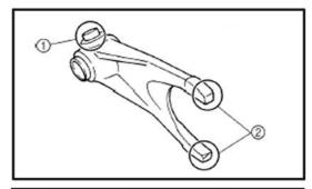
Install shift fork to guide bar and move left and right.
