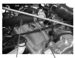
Water Outlet Hose, Engine Clamp
