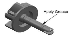
Install E-ring to water pump shaft;
