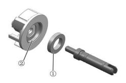
Remove mechanical seal with special tool
