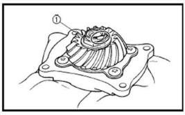
1. Drive bevel gear cover 5. Adjust washer
